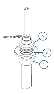
Locate the running coupler ② onto the entry ⑤ and tighten using a wrench/spanner until resistance is felt between the seal and cable, then turn the running coupler through a further half to one full turn to complete the inner seal, ensuring that entry ⑤ is prevented from turning and backnut  ${\mathbin{\textcircled{\scriptsize 1}}}$  remains tight on the conduit. This procedure compresses the seal @ into contact with the cable outer sheath.
